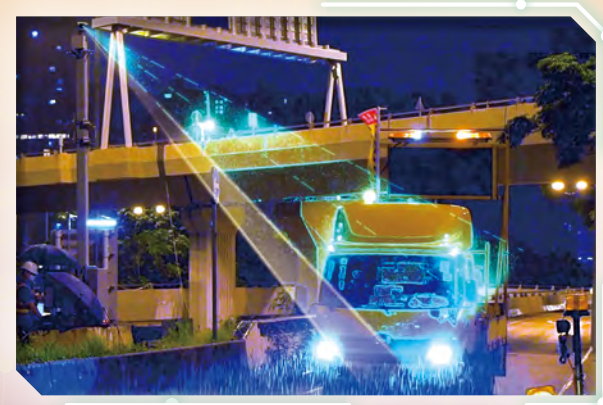
位於油麻地的光學雷達和高速相機正在掃描車輛高度和車牌號碼 The LIDAR sensor and high-speed camera at Yau Ma Tei are scanning the vehicle height and the registration mark
