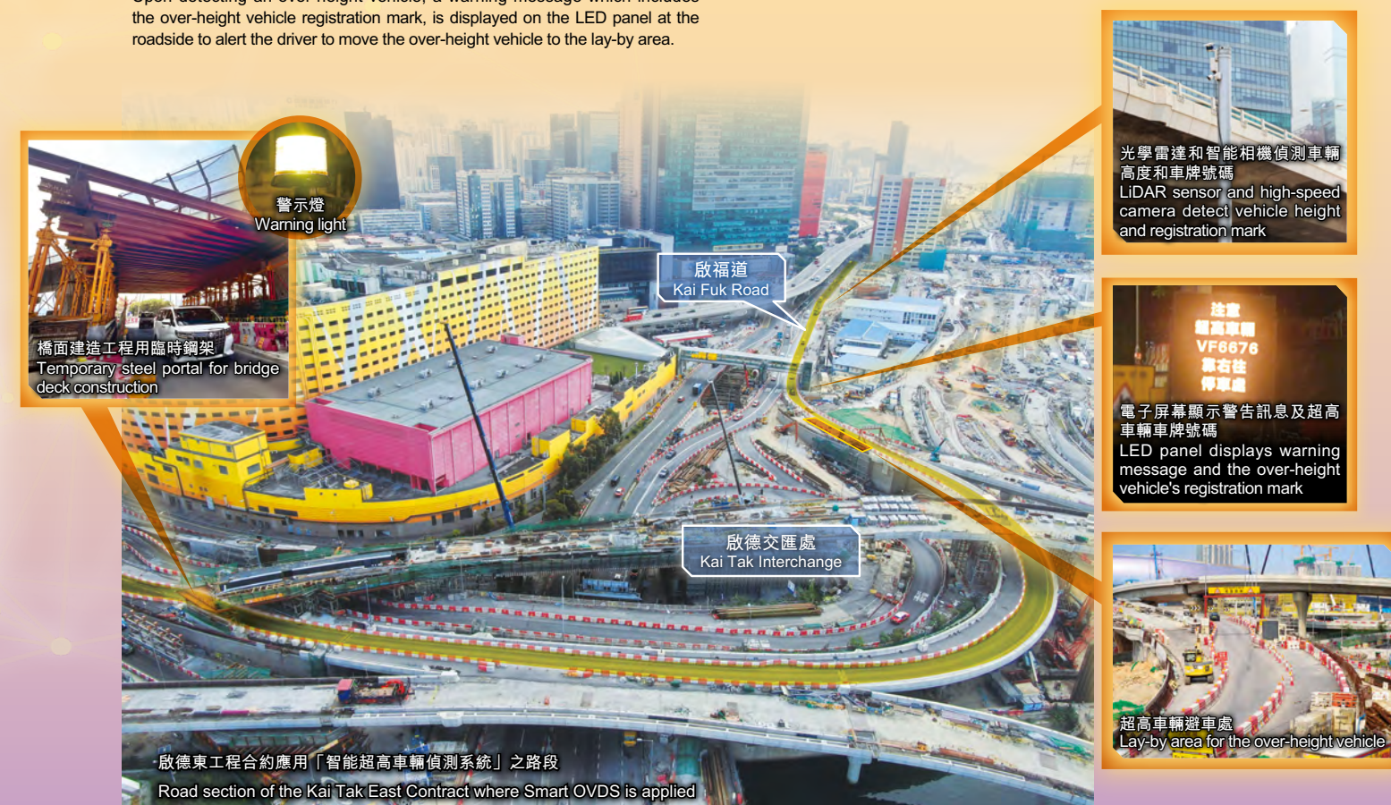
位於油麻地的光學雷達和高速相機正在掃描車輛高度和車牌號碼 The LIDAR sensor and high-speed camera at Yau Ma Tei are scanning the vehicle height and the registration mark
