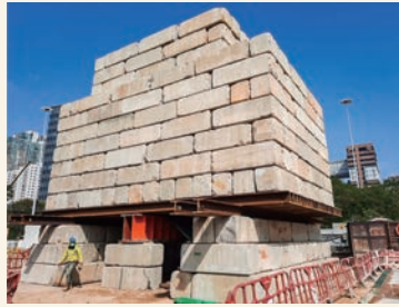
油麻地通風大樓的樁柱荷載測試 Pile load test at Yau Ma Tei Ventilation Building works site
