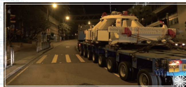
隧道鑽挖機組件由陸路運送到何文田工地 Components of TBM delivered to Ho Man Tin site by land
