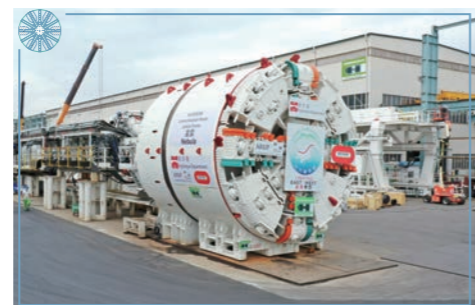
於廣州南沙廠房組裝隧道鑽挖機 Assembly of TBM at Nansha, Guangzhou
