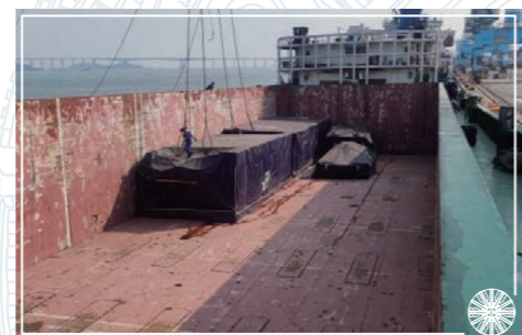
隧道鑽挖機組件由躉船運送至香港 Components of TBM delivered to Hong Kong by barge
