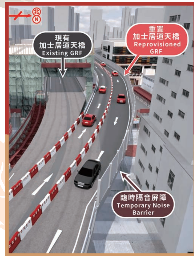
重置加士居道天橋的臨時隔音屏障 Proposed temporary noise barrier on RGRF
