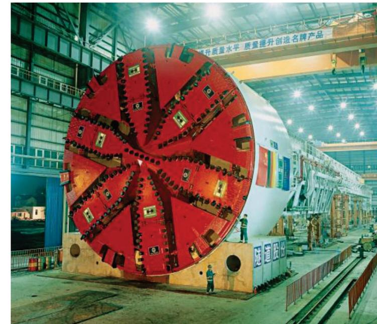
Fig. 4 Tunnel Boring Machine
