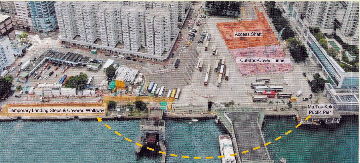
Construction of Access Shaft, cut-and-cover tunnel at Ma Tau Kok and temporary landing steps & covered walkway at King Wan Street Leisure Path
