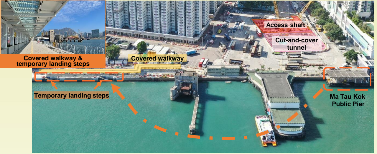
Construction of access shaft and cut-and-cover tunnel at Ma Tau Kok, and temporary landing steps and covered walkway at King Wan Street
